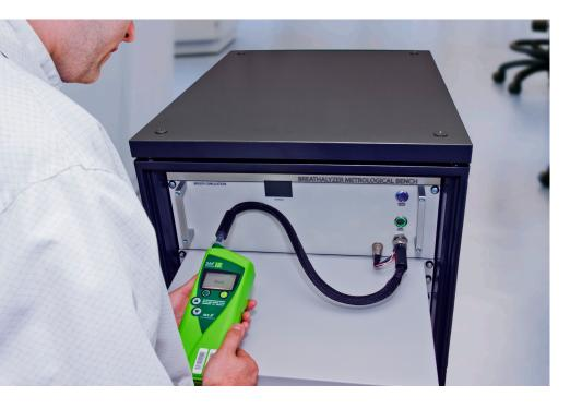
The Metrological Test Bench is designed for type testing of breath alcohol instruments against international standards and also provides the means for high volume verification testing of EBTs, where efficiency and accuracy are critical customer requirements.
