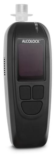
ALCOLOCK LR alcohol interlock is designed for compliance programs for drink driving offenders and prevents a vehicle from being started unless the driver provides an accepted breath sample with an alcohol concentration below the pre-set limit.
