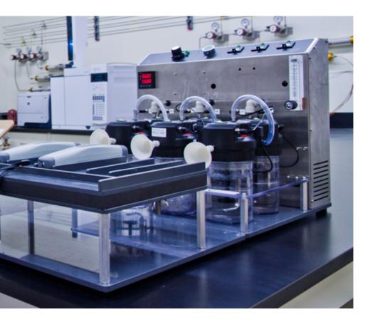
ALCOSIM calibration bench is a multi-tiered laboratory station that optimizes gas flow, alcohol reference solution use, eliminates human error and provides consistent simulated breath samples for calibration of all handheld breath alcohol testers.
