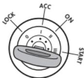
The START wire will register at +12 or +24 volts only when the key is in the "START" position
