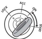
The IGNITION wire (non-continuous switched source wire) will register at approximately +12 or +24 volts only when the key is in the "ON" or "START" position
