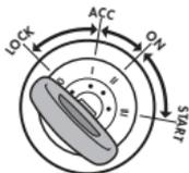
The POWER wire (continuous un-switched source wire) will register at approximately +12 or +24 volts in any key position
