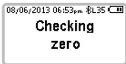
The sampling pump activates to purge the measuring chamber.
