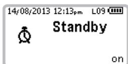
The **Standby** screen is displayed when the device is switched off and connected to a main power supply. The device can be turned on at any time while connected to a main power supply by pressing the start button
