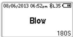
A countdown and **Blow** will be displayed. Blow into the mouthpiece with sufficient flow until the tone ends.
