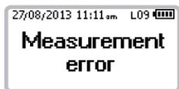
The signal is unstable and could be susceptible to punctual interference. Contact ACS or a certified service provider if the message persists.
