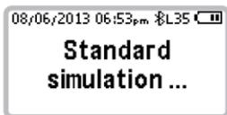
The device simulates absorption at a concentration close to the selected limit.
