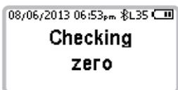
The sampling pump activates to clean the measuring chamber.
