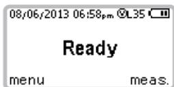
The device is now ready for a breath sample. The flashing 'v' at the top of the screen indicates **Verification mode**. To exit this mode, simply turn the device off by pressing and holding the start button
