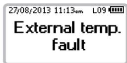
The external temperature is not within the certified range of the device (-10 to 50 °C).
