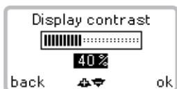
Increase the screen's brightness by pressing the *up* button ▲ and decrease with the *down* button ▼. Press the green button ● to return to the previous menu without saving or press the start button ⏻ to confirm the contrast and return to the previous screen.
