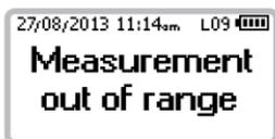
The alcohol concentration measured exceeds the instrument's operating range.
