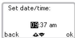
Use the *up* and *down* buttons ▲ ▼ to adjust the values accordingly.
