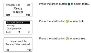
NOTE: You can also turn the device off at any time by pressing and holding the start button.
