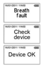
If exhalation is interrupted or if the volume is insufficient, the sampling is aborted. To restart the test, press the start button (4) to select VALIDATE
