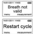
The two results are not within the range of tolerance. The test cycle must be repeated.
