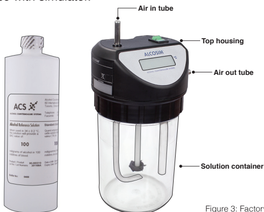
Figure 3: Factory-sealed alcohol reference solution bottle and ALCOSIM breath alcohol simulator
