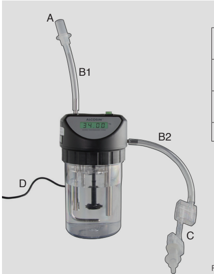
Figure 4: ALCOSIM simulator connected and ready to calibrate
