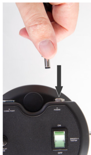
Figure 5: Connecting a power cable to the ALCOSIM simulator
