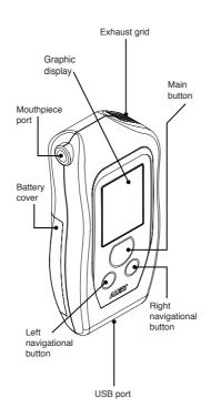
The ALERT J5 evidential breath alcohol tester is simple to use. It measures breath alcohol concentration (BrAC), which is in direct proportion to blood alcohol concentration (BAC). The readout is provided on the display.
