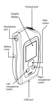
The ALERT J5 evidential breath alcohol tester is simple to use. It measures breath alcohol concentration (BrAC), which is in direct proportion to blood alcohol concentration (BAC). The readout is provided on the display.
