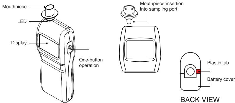
**NOTE:** In the factory, a plastic tab is inserted between the battery and the electrical connection to conserve battery power during shipment and storage. To operate the tester for the first time, pull the plastic tab from the battery compartment, which is accessible at the back of the tester. You do not need to open the back cover to remove the tab.
