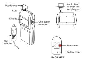
NOTE: In the factory, a plastic tab is inserted between the battery and the electrical connection to conserve battery power during shipment and storage. To operate the tester for the first time, pull the plastic tab from the battery compartment, which is accessible at the back of the tester. You do not need to open the back cover to remove the tab.
