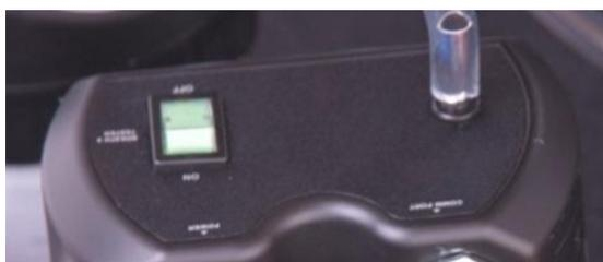
The propeller begins turning and the solution automatically begins heating up to 34°C. This takes up to 20 minutes. The ALCOSIM screen displays the temperature.
