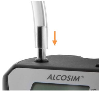
8. Connect the CS communication cable (**front**) to the ALCOSIM communication cable add-on (79-007851).
