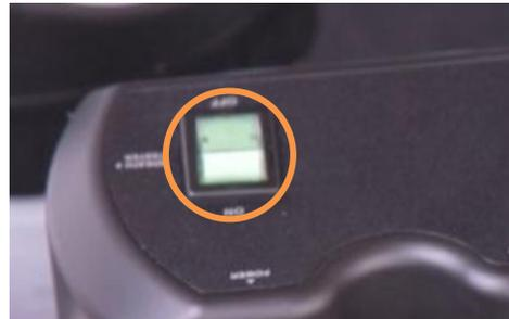
The ALCOSIM heaters and mixing propellers *automatically* activate. The ALCOSIM simulator begins heating the solution to 34°C. This takes up to 20 minutes. The ALCOSIM screen displays the solution temperature.
