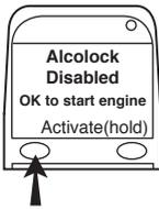
To test the display, backlights and left pushbutton: Wake the handset up by pressing the left pushbutton. The display should show, "**Alcolock Disabled, OK to start engine**".
