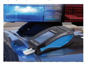
WipeAlyser is easily controlled with the integrated touch display. Entries can be made with either a finger or the supplied stylus. You will be guided through the device operation step by step. Once the prepared test cartridge is inserted into the device, analysis and reliable results are provided in seconds and read electronically.
