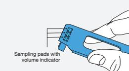
2 Without touching the sampling pads, remove the blue sample collector from the white test cassette.
