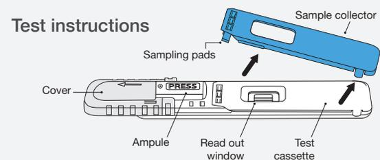
1 Slide the cover in the direction of the arrow until the word PRESS is entirely visible.
