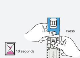
5 Hold the test cassette vertically, with the ampoule at the bottom (arrow pointing down). With your thumb, press hard on the word PRESS until the ampoule breaks. **Continue to hold for 10 seconds.**
