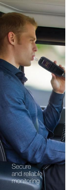
ALCOLOCK LR features an interactive handset used to perform breath alcohol tests and communicate with the driver, and an electronic unit that connects to the power and control circuits of the vehicle.
