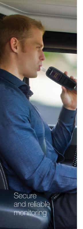
ALCOLOCK LR features an interactive handset used to perform breath alcohol tests and communicate with the driver, and an electronic unit that connects to the power and control circuits of the vehicle.
