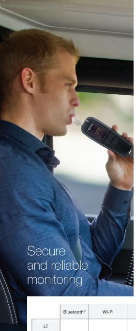
ALCOLOCK L series alcohol ignition interlocks feature a user-friendly handset to perform breath alcohol tests and communicate with the driver, and an electronic control unit (ECU) that connects to the power and control circuits of the vehicle. Drivers use the handset to provide a breath sample, and the ECU inhibits vehicle operation if the test result is above the preset breath alcohol content (BrAC) limit.
