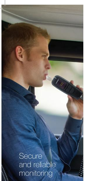
ALCOLOCK L series alcohol ignition interlocks feature a user-friendly handset to perform breath alcohol tests and communicate with the driver, and an electronic control unit (ECU) that connects to the power and control circuits of the vehicle. Drivers use the handset to provide a breath sample, and the ECU inhibits vehicle operation if the test result is above the preset breath alcohol content (BrAC) limit.
