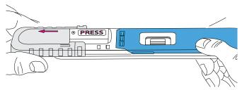
3 Remove the blue sample collector from the white test cassette, **without** touching the sampling pads.
