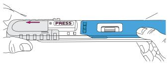
Remove the blue sample collector from the white test cassette, **without** touching the sampling pads.
